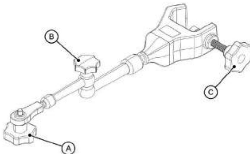
1. Extract the “EU2511 Ecmlife holder motor driver” from the package and use the central knob (A) to loose or tight the holder in the desired position
