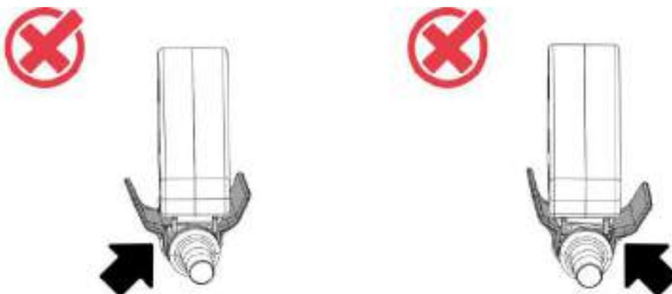
Remove venous probe from cuvette by pressing the retaining tabs with the fingers. The retaining tabs will expand releasing the probe.
