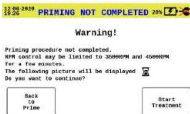
In order to reach an RPM set-point higher than 3500RPM and 4500RPM it's necessary to allow the device to perform a two minutes of calibration in a range between these two target.
