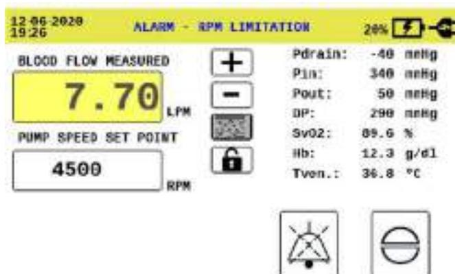
When 3500 RPM or 4500 RPM setpoint is reached, the calibration will be performed by console by remaining for at least 2 minutes in a range within 1550RPM-3450RPM for the first self-learning setpoint and 4300RPM-4450RPM for the second self-learning setpoint.
