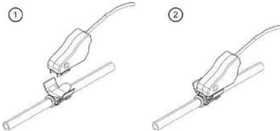
Venous probe correctly installed onto the cuvette
