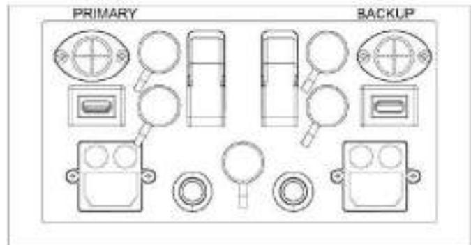
3. Ensure the ECMOLIFE-COLIBRÌ cable to the dedicated socket of ECMOLIFE connector panel.
