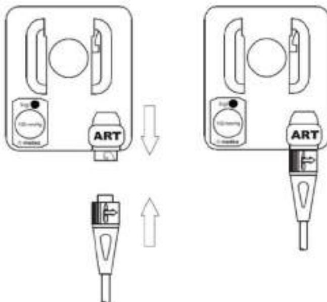
Insert the cable to the relevant pressure connector (Pin – Pout –Pdrain) on ECMOLIFE console. For the assembly of Single use MEDEX (Smith Medical) pressure transducer refer to relevant instructions for use.
