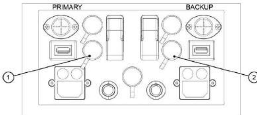
In order to avoid any electrical interference between ECMOLIFE device and ambulance on board systems The dedicated Ambulance Power Module interface EU3953 must be used.
