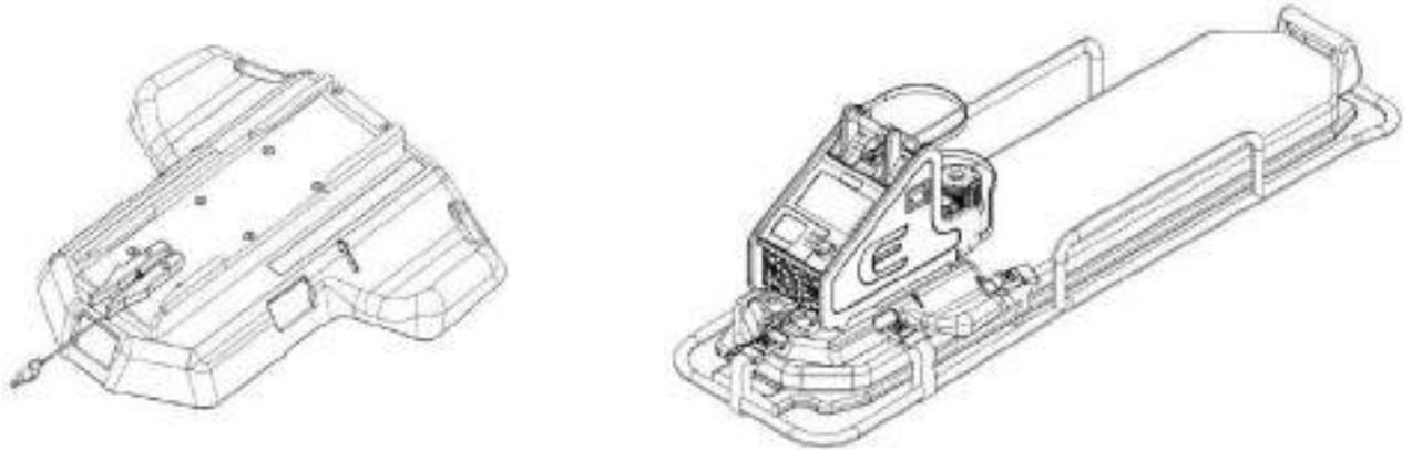
FOIL STRETCHER HOLDER PLATE EU3996 is conceived to safely support and transport the ECMOLIFE CONSOLE during road ambulance transport through a dedicated interface which can be located between the legs of the patient.
