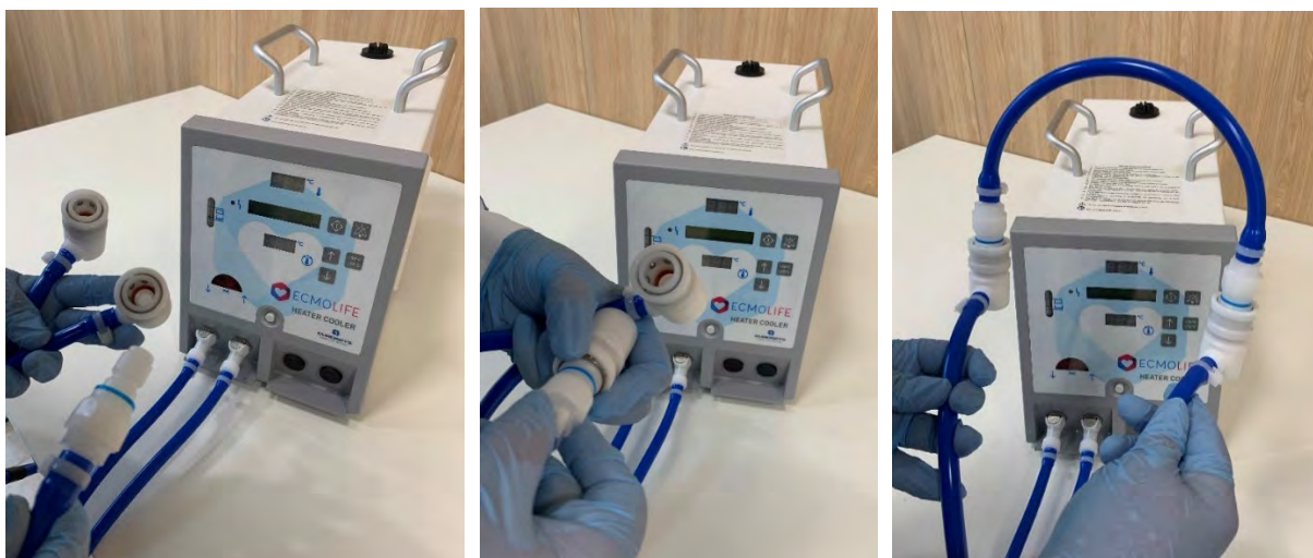
Figure 24 - Connection of Hansen connection tube to hoses
